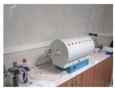
EN 50267-2-3:1999 / BS EN 50267-2-3:1999 / DIN EN 50267-2-3:1999 / VDE 0482-267-2-3:1999-04 / CEI EN 50267-2-3:1999 (CEI 20-37/2-3). Common test methods for cables under fire conditions- Test on gases evolved during combustion of materials from cables-Part 2-3:Procedures. Determination of degree of acidity of gases for cables by determination of the weighted average of pH and conductivity.
